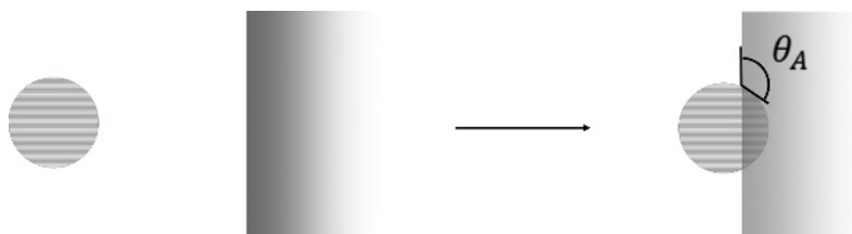
Figure 1.7 A hydrophobic, spherical particle moving from the air to a position in a water interface where it has its contact angle with the liquid.
